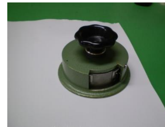
GSM Test (Measures the Weight)
