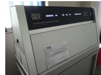
QUV Tester (Accelerated Weatherometer, mimics Sunlight, Rain and Dew)
