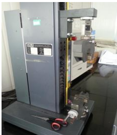
Fabric Tensile (Tensile, Compression, Shear, and Peel)
