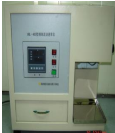
MFI Tester Melt Flow Indexer (Polymer Testing Machine)
