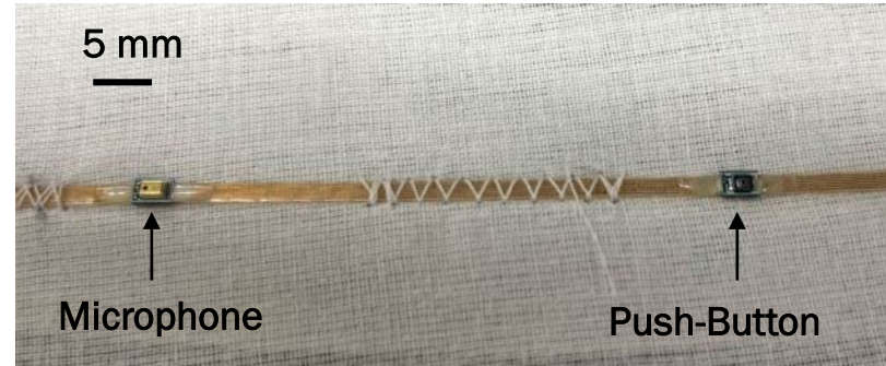
Audio baseline electronics includes five nodes embedded in a polymer fiber
