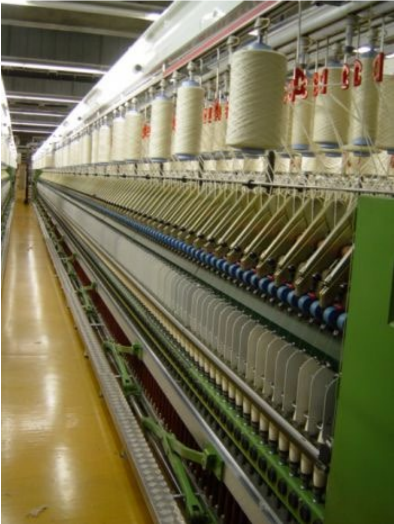
Worsted Spinning and Twisting Plant with 20,500 spindles
