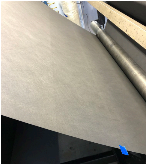
Hot calender roll engaged and disengaged during at 67 yard mark during base nonwoven manufacture .....
