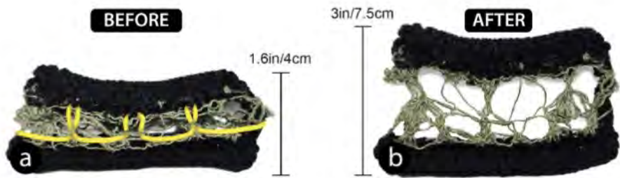
Figure 4: "Unfolding Lace Top" swatch to test the unfolding stitch structure. a. before, and b. after dissolving the swatch in cold water.
