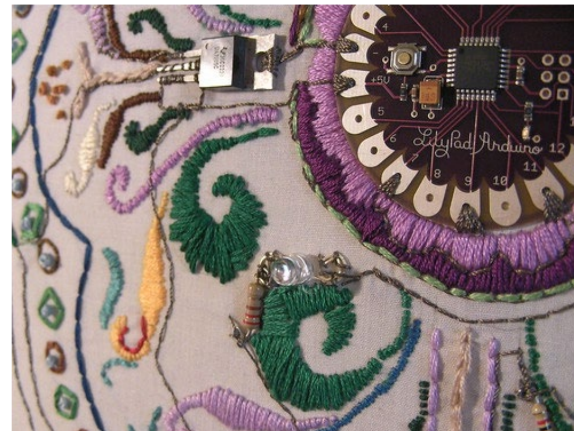
Fabric PCBs: e-textile craft Buechley and Eisenberg, UbiComp (2009).
